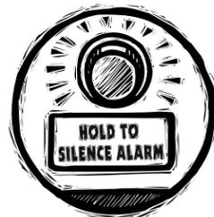
**Do** remember that the audible alarm can be silenced by pushing the lighted button located directly above the "Push to Silence" label on the front of the electrical control panel. Hold the button until the alarm goes off. With normal use, the tank has a reserve storage capacity good for about 24 hours.
